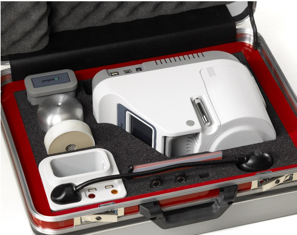
Fig.3. Pegasor AQ Indoor in a suitcase
