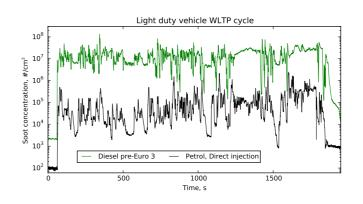
Pegasor PPS-G2 sensor used in GDI engine and pre-Euro3 diesel engine measurements demostrates the wide dynamic range and capability of the measurement technology.
